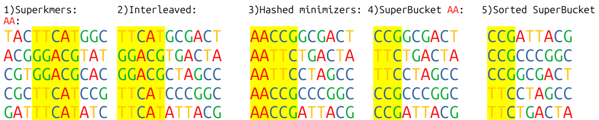
Figure 13.3.: Construction steps of a superbucket. Minimizers are highlighted in yellow. Plain super- k -mers (1) are rewritten in interleaved form (2), the minimizer is replaced by its hashed value (3), the common superbucket prefix is made implicit (4), and the list is sorted (5).
